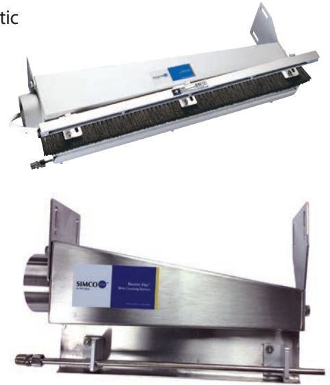
Neutro-Vac Brush Contact Head with Static Bars & Air Tube (available without a brush as a non-contact version)
